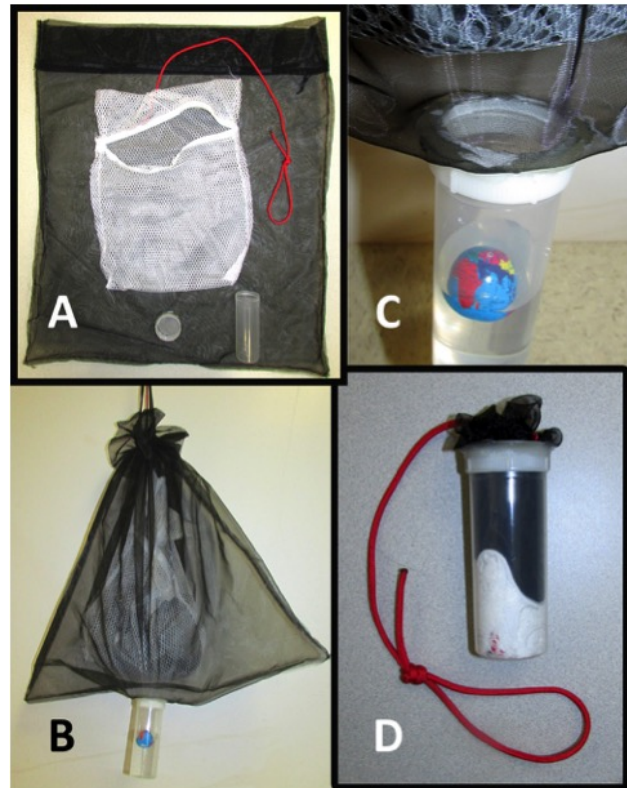
Figure 1. A Winkler sampler lets you collect a world of possibilities! (A) all the parts apart; (B) sampler engaged; (C) close-up of collection vial, outer organza bag, and inner sample bag; (D) sampler stuffed into the collection vial.
