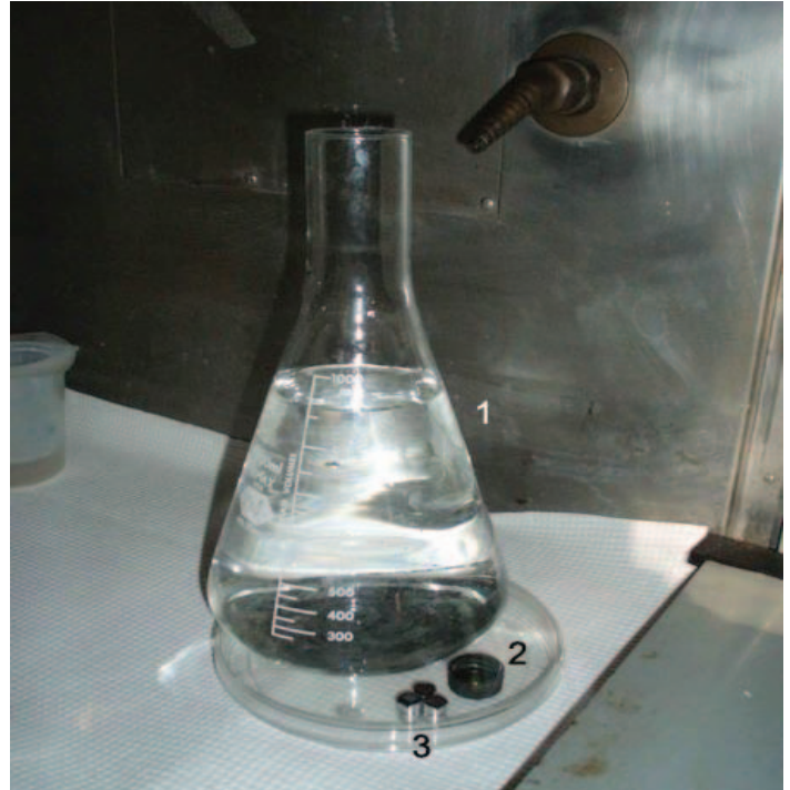
Fig. 1. Example of vapor-coating apparatus. 1, beaker or Erlenmeyer bottle with hot water; 2, bottle cap with coating metal; 3, stubs with specimens to be coated.
